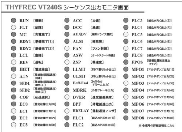
Fig. 11 Sequence I/O Signal Monitor Screen You can see the ON/OFF status of inverter I/O sequence signals on the screen.
