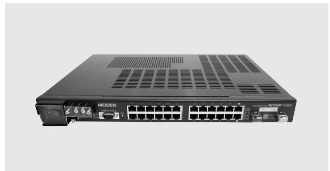
Fig. 2 L3 Switching Hub, MEISWAY TW900
