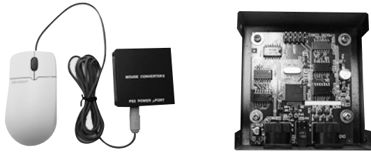
(a) General-purpose PS2 mouse and its replacing adapter (b) Inside of replacing adapter
