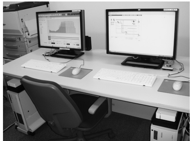
Fig. 5 Operator Console for the Smart BEMS
