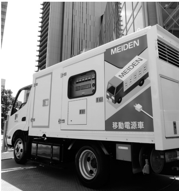
Fig. 4 Mobile Genset with Total Vehicle Weight of Less than 5 tons
