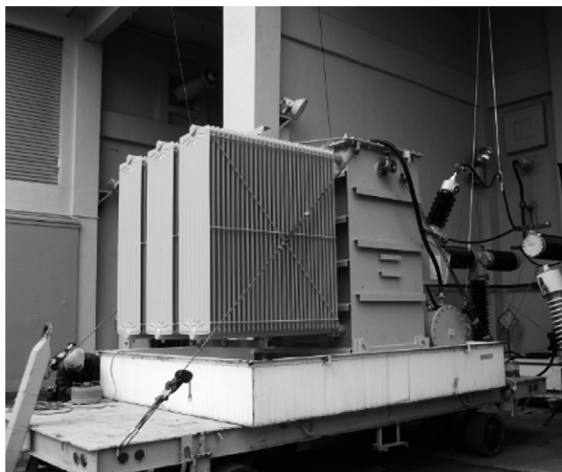
Fig. 3 Situation of Short-Circuit Testing
