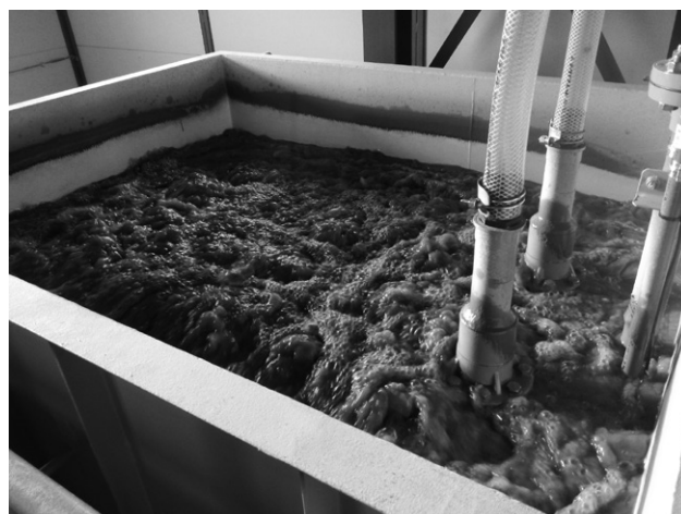
Fig. 6 Example of Field-Testing for Immersion Type Membrane Modules in Membrane Separation Tank (SS = 2700mg/L)
