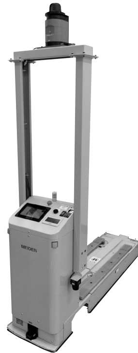
Fig. 3 Lift-Type Low-Platform AGV Introduced at Electronic Component Assembly Line
