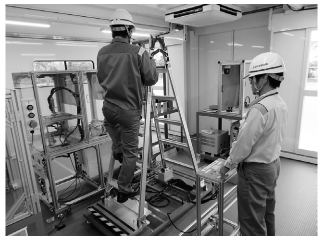
Fig. 7 Stepladder Wobble Experience Device
