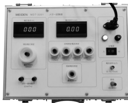
Fig. 10 Operation Panel of Megger Tester
