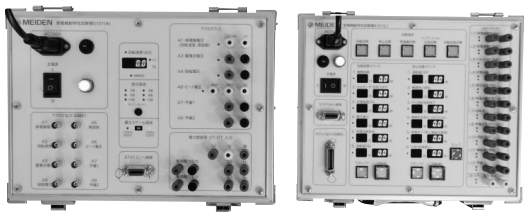
Fig. 12 Operation Panel of Generator Dynamic Characteristic Tester
