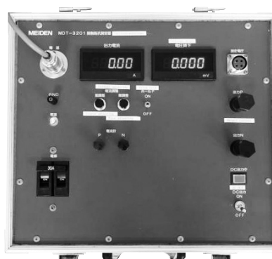
Fig. 11 Operation Panel of Contact Resistance Measuring Instrument
