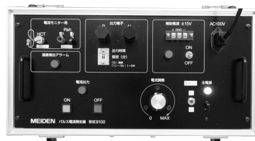
Fig. 14 Operation Panel of Pulse Current Generator
