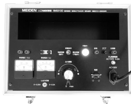
Fig. 13 Operation Panel of Artificial Ground Fault Tester
