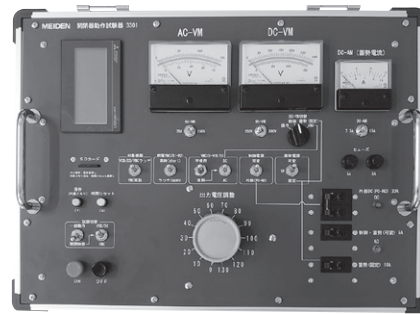
Fig. 1 Operation Panel of Switching Device Operation Tester
