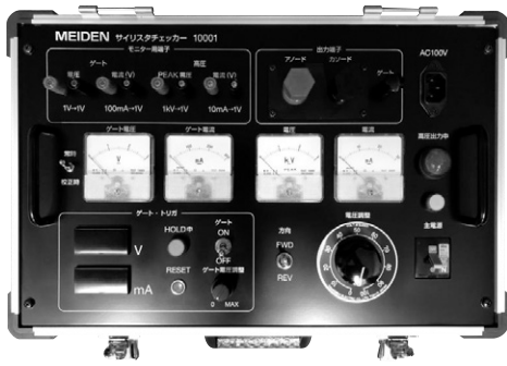
Fig. 4 Operation Panel of Thyristor Checker
